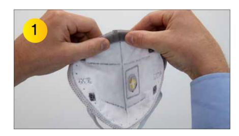
Using both hands, place fingers and thumbs on underside of nosepiece. Unfold respirator by pulling both side panels out so the respirator is fully unfolded to form a cup shape.
